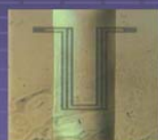
GaAs membrane supported coupled line filter for 45 GHz
